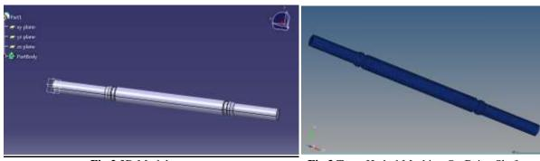
Fig.2 3D Model Number Of Nodes: 3937 Number Of Elements: 15858 Element Size = 4 Mm
