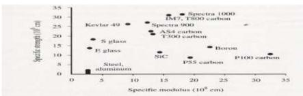
Fig 8 Specific Modulus And Specific Strength For Various Engineering Materials And Fibers (Swanson S.R; 1997; 3)
